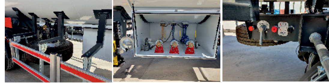
52 m³ P460 STEEL LPG SEMI TRAILER TANK
